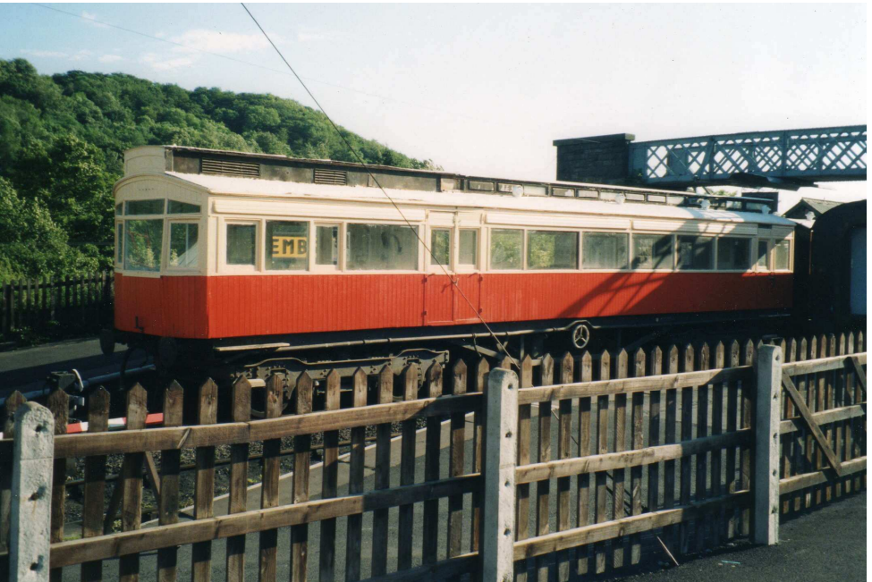
Above; From the archive, a quiet spell at York for an autocar in the early 1900's. Below; 3170 moved to Embsay in 2003 and was placed on an accommodation under-frame from a Gresley carriage. Seen here repainted in its original NER red and cream colours for publicity purposes. Photo S Middleton
